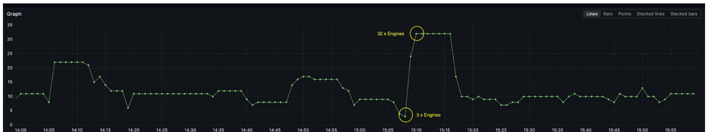
Figure 6: An example of a single cloud region engine auto-scaling on a typical day
